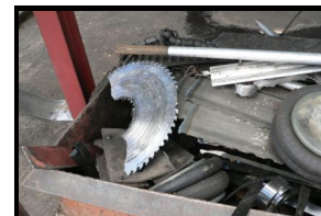
Scrap box. Check out saw blade ripped in half during milling
