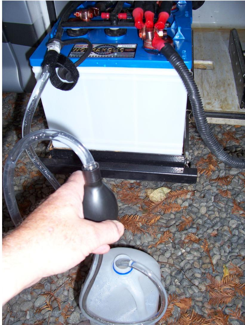
In asking around, we have found that many savvy owners, not only of motor coaches, but of all sorts of other equipment that depends upon wet cell batteries for power, use this clever system to maintain the proper level of electrolyte in their batteries.
