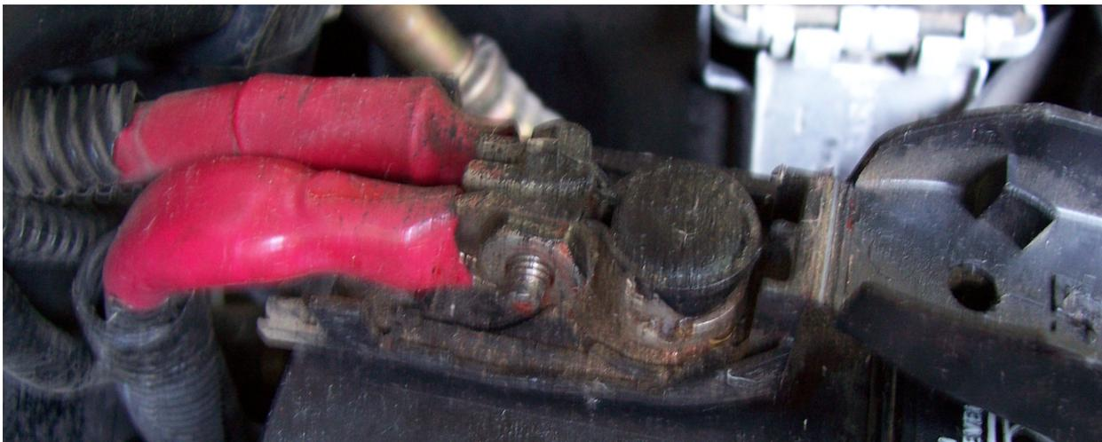
Because we were totally unaware that this connection was not tight, the chassis battery was discharged completely and repeatedly, quickly leading to its expensive demise.
