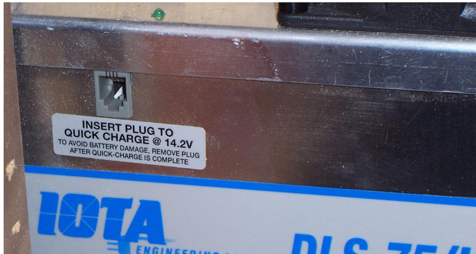
Needless to say, because of its inaccessible location and the fact that there was no information about it in our Owner's Manual, no one had ever removed it! No wonder we had boiled our batteries! I immediately removed the jumper plug, and we are happy to report that we have not boiled a battery since, and the water levels in the world's oceans has stopped going down since we are no longer consuming so much distilled water.
